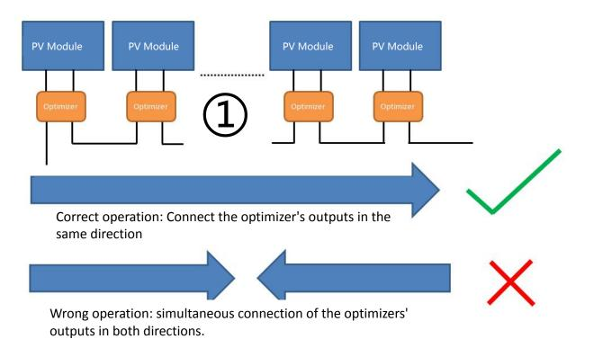
Description: When all the inputs of the optimizers are connected to the output of the PV junction boxes, the outputs of the optimizers are connected in series.
