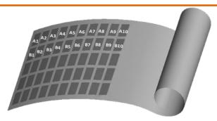
②. Use a screw or cable tie to position the optimizer or PV monitor one by one according to the registered MACID number position, and fix it on the bracket or panel frame. If the bracket has no mounting holes, it can be drilled and mounted with a hole size of 6mm.
