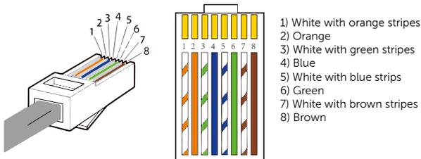
The steps for making RJ45 connector to BMS communication cable (Part A) are shown as follows:
