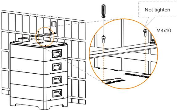
Move the assembled bracket to the wall;
