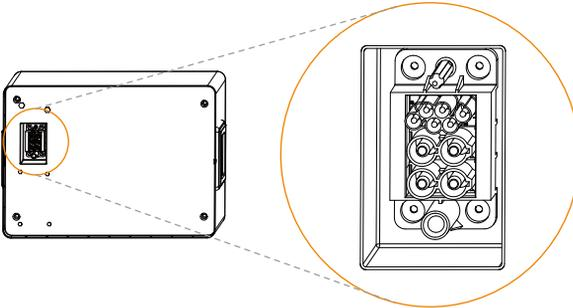
The hot-plug interface is connected to the top of battery module or Base.
