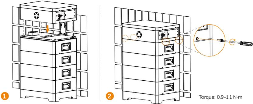
\*Note: Regarding the cover plate on both sides of the BMS, they should be installed after finishing wiring.
