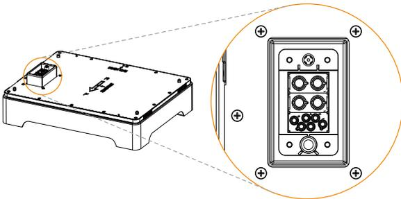
The hot-plug interface is connected to the bottom of battery module.
