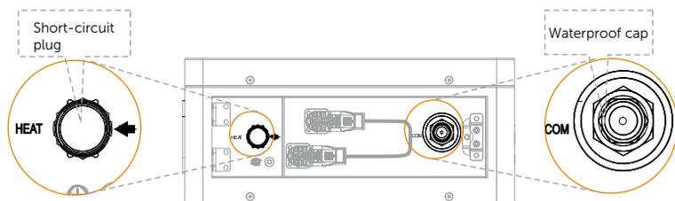
\*Note: In case of one tower, a waterproof cap shall be put on the unconnected "COM" port, as well as a short-circuit plug on the unconnected "HEAT" port.
