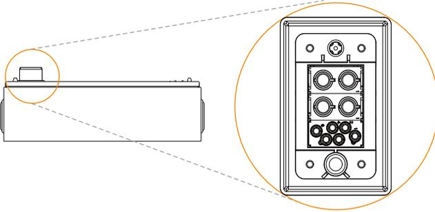
The hot-plug interface is connected to the bottom of battery module or BMS.
