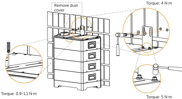
Step 8. Place BMS, and tighten M4x14 Phillips-head screw (Part L) (x 4 pcs) and gasket (Part K) (x 4 pcs) on both sides (Torque: 0.9 to 1.1 N·m)
