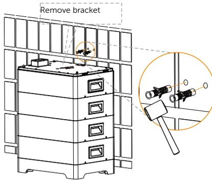
Secure the assembled bracket to the wall with Self-tapping screw (Part H) (x 2 pcs) and Washer (Part G) (x 2 pcs), and tighten them (Torque: 4 N·m);
