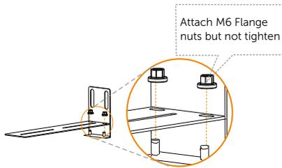
Step 7. Secure the assembled bracket on the battery module and wall.
